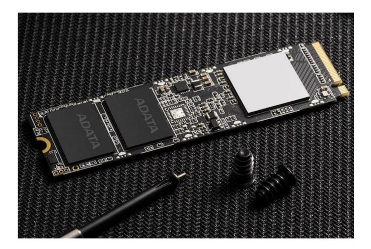
The aforementioned controller allows for features including 8 NAND channels, PCIe 3.0 x4 and NVMe 1.3, among others. The drive is built using 3D TLC NAND, and offers performance clocking at 3.5GB/s in sequential read and 3GB/s in sequential write. Random performance totals 300L/240K in random read/write, while IOPS is at 4K.
