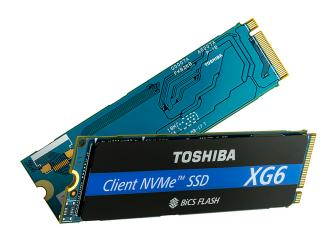
The drives will find a variety of uses across the client PC, high-performance mobile, embedded and gaming segments, as well as datacentre environments for boot drives in servers, caching and logging, and commodity storage. They are available in an M.2 2280 single-sided form factor, with support for PCIe Generation 3x4 lane and NVMe revision 1.3a.
