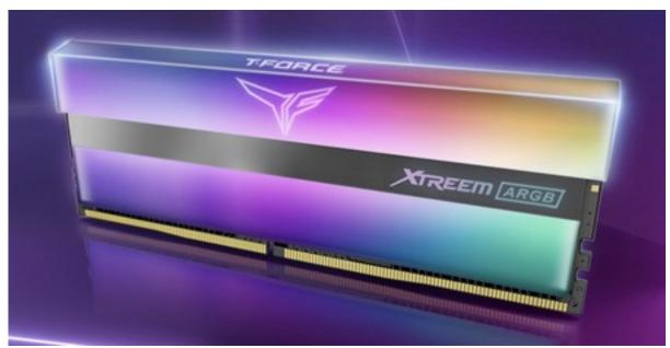
The mirrored heat spreaders allow the memory modules to reflect the light emitted by the RGB LEDs inside the lightbar on top, illuminating the entire surface of the module. Teamgroup says it is the result of a mixture of "light-spluttering" and light guiding technology, and makes for a more striking effect than the lighting strips found in typical gaming memory modules.
