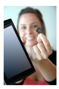
SanDisk's new SSD, smaller than a postage stamp and weighing less than a Euro cent, comes in capacities from 4GB to 64GB. This iSSD is fast enough for use with advanced operating systems such as Windows 7 or Mac OS X
