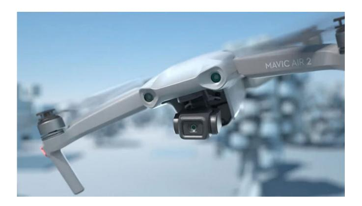
Featuring the same portable foldable design as the first model, the Mavic Air 2 weighs 570g and carries updated motors, new electronic speed controllers (ESCs) and an enhanced battery allowing for up to 34 minutes of flight. Proprietary OcuSync 2.0 connectivity provides a reliable and stable video feed from the drone at a maximum distance of 10km. The connectivity technology supports both 2.4 and 5.8GHz frequency bands, and auto-switches between the two according to signal strength.
