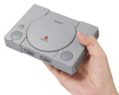
The PlayStation Classic is 45% smaller than the original machine and retains the same stylings, down to the circular power, open and reset buttons. Meanwhile the controllers are replicas of the originals. They connect to the console via cable, allow for local multiplayer gaming and lack analog sticks.
