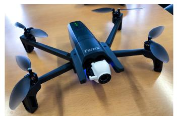
Named after the Greek island, the Anafi carries a 21MP camera on a 180-degree tilt gimbal able to record 4K HDR video at 30fps (or 1080p video at 60fps). The extra resolution sensor allows for lossless 2.8x or 1.4x digital zoom when recording in HD and 4K, respectively. Further camera features include a hyper-lapse mode allowing one to speed footage up to 240x, slo-mo and a high frame rate mode up to 60fps. Video and photo storage comes on microSD card.
