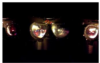
The Half Dome increases field of view from the 110-degree offered by the Oculus Rift and HTC Vive to 140-degrees. Thus, users can view more of the virtual world, even as the prototype retains the same dimensions as the existing Rift headset. Oculus says such a development comes through "continued advances in displays," something it will continue to work on before shifting focus on shrinking the headset.
