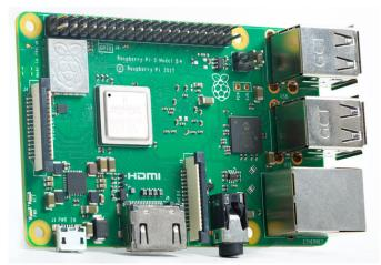
The Model B+ runs on a Broadcom BCM2837B0 64-bit quad-core ARM Cortex-A53 CPU-- the same processor as the regular Model B, only clocked at a faster 1.4GHz. It also promises "power integrity optimisations and a heat spreader" allowing customers to either overclock the little machine or run it at lower voltages to reduce power consumption. Interestingly the maker says the B+ consumes "substantially more power than its predecessor," and recommends the use of a high-quality 2.5A power supply.
