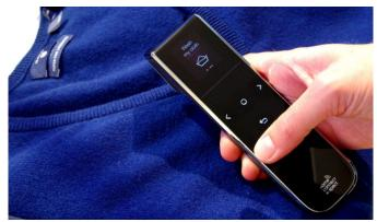
Dubbed the X-Spect, the handheld device looks like a TV remote and comes complete with a small screen and capacitive touch buttons. It essentially scans fabrics and stains before suggesting how to best wash the garment in question. An IFA demonstration even had the X-Spect paired via wifi with a Bosch washing machine, allowing it to send optimal washing instructions.
