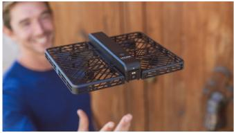
Developed by Zero Zero Robots, the Hover Camera Passport is a foldable drone built from carbon fibre material. It weighs just 242g and carries a 13MP camera with 4K video support and the ability to capture 360-degree panoramic video. Battery life clocks at around 10 minutes per charge, and the makers promise the Passport is very easy to use, with artificial intelligence allowing anyone to operate both indoors and outdoors.
