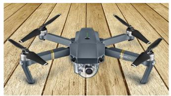
The Mavic Pro does not exactly qualify as palm-size, but is small enough to fit in a backpack or purse when folded. Sensors on the front and bottom provide obstacle avoidance, subject tracking, autonomous landing and indoor stability, while a 12MP camera sensor shoots 4K video at 30fps and HD video at 96fps.
