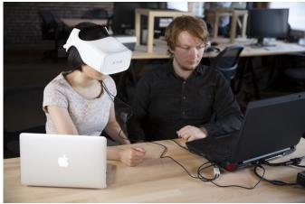
The headset, also dubbed Fove, promises superior interaction with virtual worlds, since the human eye is actually fast, accurate and very responsive. Said tracking is done through the combination of a pair of infrared cameras and an appropriate algorithm.
