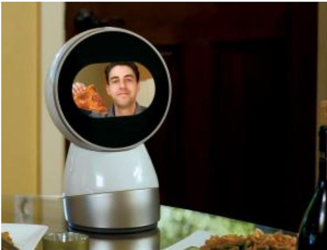
Looking like something out of a slightly sinister science fiction movie, Jibo is essentially a pod on top of a 3-axis motorised swivel. The pod carries dual cameras, 360-degree microphones, a 5.7-inch circular display, a quad-core ARM processor and wifi radios, as well as software handling artificial intelligence, facial recognition and natural language processing.
