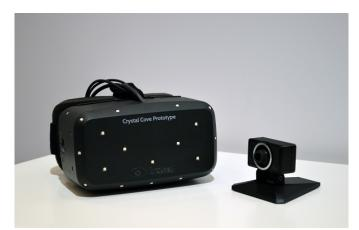
The updated AMOLED display handle 1920x1080 resolution and features low persistence, a technology reducing the picture smear and motion blur causing motion sickness to at least some users. Meanwhile latency is down to around 30ms, meaning Oculus is getting closer to its aim of sub-20ms latencies.
