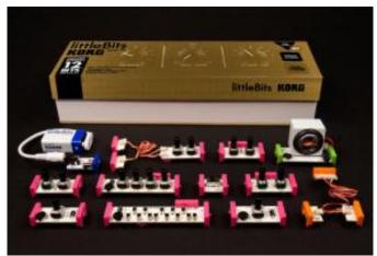
The kit contains 12 modules-- 2 oscillators, envelope and filter units, keyboard, 4-step sequencer, random noise generator, 2-channel mixer, delay effect, power source and speaker. Each component is colour coded (blue for power, pink for input, green for output, orange for wire) and carries magnets on either side for easy snapping in a specific direction.
