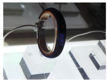
Just like those devices, the LG Smart Activity Tracker tracks fitness habits (via accelerometer and altimeter) once paired with a smartphone carrying a companion app. Nike+ FuelBand users will also be familiar with the dotted LED display, USB clasp and soft-touch rubber coating.
