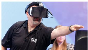
Described as "the future of merged reality" back at its 2016 Intel Developer Forum reveal, the Project Alloy headset carried all components to power VR experience. As such, it allowed a full range of motion with 6 degrees of freedom (6DoF), as well as Augmented Reality (AR) via RealSense technology.
