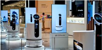
Developed by the LG lab responsible for a number of robots released under the CLOi brand, the shopping cart robots promise to "free visitors from the hassle of pushing heavy carts by themselves." The company says the robots will follow shoppers as they walk through the aisles, automatically avoiding obstacles along the way.
