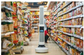
The idea behind Tally is pretty straightforward. One or more Tally units roam around brick-and-mortar retail environments to keep track of the merchandise available on the shelves. The robots detect out-of-stock and low stocks, identify misplaced or incorrectly facing items and even validate price tags, all with vendor management and 3rd party supplier compliance.
