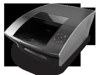
The secret lies in what Memjet calls Waterfall Printhead technology-- printing through a single fixed 8.77" printhead covering the entire width of an A4 sheet of paper with 70400 nozzles (x17 the amount in a regular inkjet) to deposit 774 million dots of ink per second. Being stationary, the system improves performance while reducing the noise, vibrations and mechanical complexity of traditional inkjet architectures.
