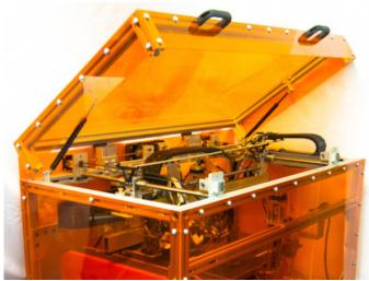
"Multi-material" 3D printers already exist, if in the shape of industrial machines able to print able to use up to 3 materials at a time. The Multifab claims to be superior to such devices through the use of 3D scanning and machine vision technologies.
