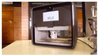
The work of Barcelona-based Natural Machines, the Foodini uses the same technological principles as regular 3D printers. Obviously, instead of plastic filament it uses raw ingredients (as deployed via stainless steel capsules), which it prints out, layer by layer, until it forms food.
