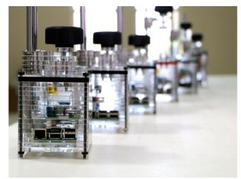
How small is the iBox Nano? All of 10 x 7 x 20cm. Makers iBox Printers say such dimensions are possible through use of liquid resin instead of plastic filament for 3D printing, which the printer hardens layer by layer via UV LEDs. Further shrinking the printer is construction in laser-cut extruded acrylic (aka Polymethyl metacrylate or PMMA).
