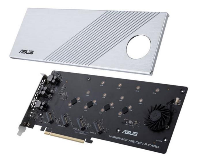
The card offers four M.2 slots, each with four lanes of PCIe 4.0 connectivity. The slots are diagonally positioned, allowing the flexibility to fit 2242, 2260, 2280 and 22110 form factor (the first two digits denote width, the following digits length in mm) M.2 cards. In turn the card supplies up to 14W of power to each M.2 SSD, enough to run the storage devices "at full potential," at least according to Asus.
