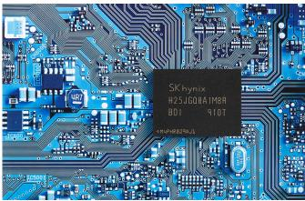
According to the company, the chips feature the application of QLC technology to a 96-layer CTF (Charge Trap Flash) based on 4D NAND flash. QLC stores 4 bits of data in one NAND cell, allowing higher density compared to TLC (Triple Level Cell) with 3 bits per cell. Furthermore, SK Hynix says the product has reduced the area to less than 90% of of existing 3D-based QLC products.
