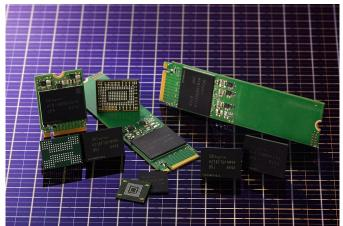
A single 512Gb NAND flash chip can represent up to 64GB of storage. As the company puts it, the combination of 3D CTF with PUC is an industry first, and allows for the finest performance and productivity yet.
