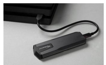
The Savage EXO SSD is available in 480 or 960GB capacities, and offers read speeds of up to 500MB/s and write speeds of 400MB/s. It comes in a compact form factor measuring 123.82 x 48.61 x 10.24mm and weighing just 56g, and is compatible with Windows and Mac PCs as well as Xbox One and PS4 consoles. Connectivity comes via USB-C interface.
