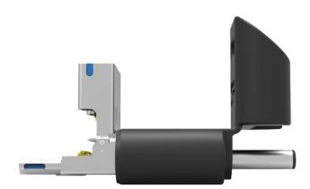
The standard Type-A connector with one side up is found at one end. Users can lift up the Type-A connector to reveal the Micro-B connector for older phones and tablets. On the other end, hidden under an elastic black cap, is the Type-C connector for modern devices.
