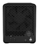
According to the company, Thunderbolt 3 connectivity also allows users to connect a pair a 4K monitors (or one 5K display) to the 5D3, or daisy-chain up to 6 Thunderbolt 3 devices, all with enough power to (slow) charge a laptop. It has two Thunderbolt 3 ports, together with a USB-C port.
