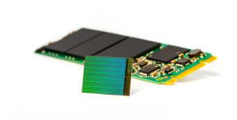
According to the company 3D NAND is a solution for the cramming of more storage capacity within a smaller space. The concept behind the technology is actually reminiscent of a skyscraper, since it involves stacking memory cells on top of each other-- and the higher the memory cells go, the more storage is available.
