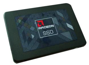
Manufactured by Taiwanese OEM Galt, the Radeon R3 SSDs come in a 2.5-inch form factor, are 7mm thick and are compatible with the SATA III 6GB interface. Inside are TLC NAND and a Silicon Motion M2256KX controller.
