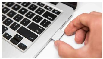
What makes the Pear different from other SD card products is software "merging" the SD card with the MacBook SSD, creating unified storage volume users can tap into like a regular built-in drive.
