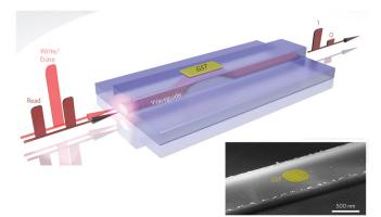
According to the researchers electronic data exchange between processors and memory limits the speed of modern computers. This is due to the electrons running through the metal wires making the logic circuits inside computer chips bumping into each other, slowing down and generating heat. Optical technology does not have such problems, as photons (the particle making light) travel well together at, well, light speed.
