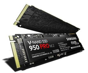
Available in 256 and 512GB sizes, the 950 Pro features 2nd generation 32-layer V-NAND and Non-Volatile Memory express (NVMe), a protocol designed to further improve SSD performance through reduced power consumption and longer-lasting use. As such, Samsung warranties the 512GB model to write up to 400TB of data.
