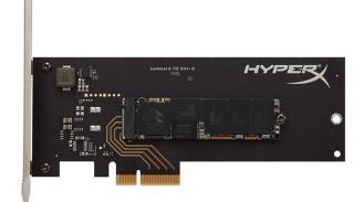
The Predator SSDs feature a PCIe generation 2x4 interface in M.2 form factor, and HyperX offers optional half-height, half-length (HHHL) adapters with both standard and low-profile brackets to fit slim desktop builds. Powering all is a Marvell 88SS9293 controller
