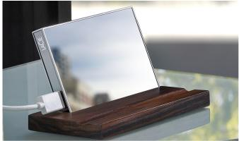
The LaCie Mirror is an external HDD with a rather self-descriptive name-- after all, the USB 3.0 storage device is covered in mirrored Gorilla Glass, making it reflective as well as rugged and scratch-resistant.
