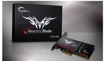
It features x4 LSI SF-2281 SSD controllers in a RAID0 setup and integrated 480GB MLC flash array, promising a bandwidth performance increase of up to 4 times over SATA3-based SSDs. Read and write speeds reach up to 2000Mb/s, while performance clocks at up to 245K IOPS with 4KB random write.
