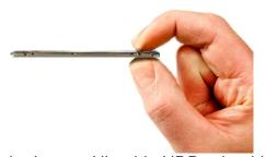
Seagate ships the Laptop Ultrathin HDD-- the thinnest 500GB HDD from the storage maker yet, with a 5mm profile designed for use in the slimmest of notebooks and tablets.
