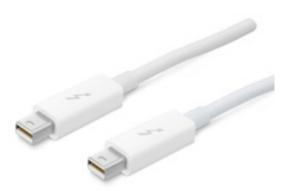
Using x5 copper wire pairs (2 handling uploads, 2 handling downloads, 1 for side channel traffic) over PCI-E (on motherboard) and DisplayPort, Thunderbolt carries up to 10Gbit/s of bidirectional data transfer-- 2x faster than USB 3.0 (or 12x faster than FireWire 800).
