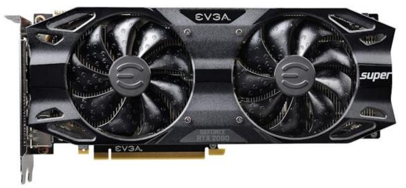
The two Super KO models include a dual-slot, dual-fan cooler within a black-themed design lacking in any RGB LED lighting. Also lacking is the backplate, while I/O comes through triple DisplayPort 1.4 and one HDMI 2.0 outputs. The RTX 2080 models has the same specifications as the Super Founders edition, with base clock speed reaching 1650MHz, boost clock of 1815MHz and 8GB of GDDR6 memory clocked at 15.5Gbps over 256-bit memory bus.
