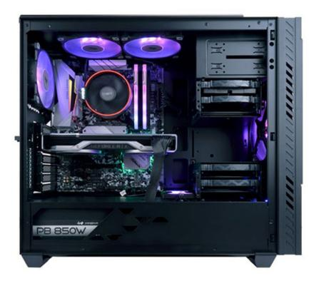
First seen back at CES 2020, the C200 lacks the frills typical of PC hardware aimed at the gaming market. It is built using strong SECC steel side panels, and features large thumbscrews for the easy removal of panels. In total, the case has space for up to six 3.5-inch HDDs (customers can convert the drive cages to SSDs) and two 2.5-inch SSDs, plus two 5.25-inch drive bays ideal for ODDs or up to three front-accessible hot-swappable HDDs.
