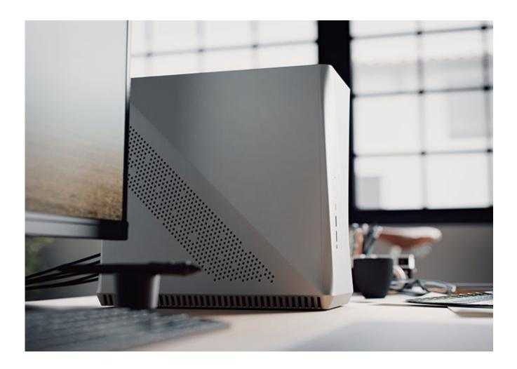
Designed in collaboration with Intel, the Era ITX features a surfaced aluminium exterior and top inserts in a choice of different materials, including wood and tempered glass. While small, Fractal Design says a flexible PSU mounting system allows the case to carry a 9th gen Intel Core processor together with a dual-slot GPU, AIO water cooling unit (up to 240mm) and up to x4 storage devices.
