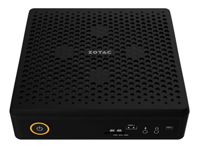
The Magnus EN92080V chassis is just 62.2mm tall, and carries an 8-core Intel i9 processor (with 45W TDP) and the laptop version of the Nvidia GeForce RTX 2080 graphics processor. it can also house up to 32GB of DDR4-2666 memory in two SO-DIMM slots as well as one 2.5-inch storage device and an M.2 SSD.
