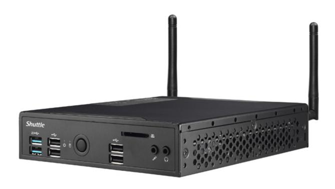
A successor to the DS77 series, the DS10 range consists of the DS10U, DS10U3, DS10U5 and DS10U7. Processor options range from the Celeron 4205U inside to the DS10U to the Core i7-8565U in the DS10U7. All come inside a 1.3I steel chassis offering silent fanless performance, and are designed for 24/7 operation with passive cooling allowing less dust to enter the insides.
