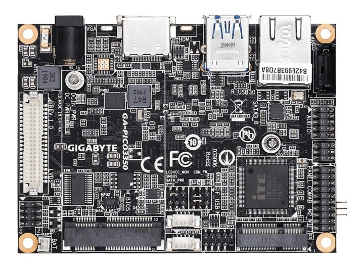
The 6W processor is soldered on, and offers 2C/2T with a base boost of 1.1/2.4GHz. In addition, the motherboard has a single SO-DIMM with support for up to 8GB of DDR3L memory running at 1600/1866MHz, and offers dual-display capability through 24-bit dual-channel LVDS with max resolution reaching 1920x1200.
