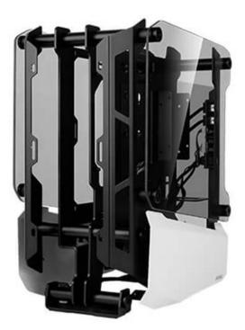
The Striker chassis consists of an aluminium and steel structure holding a pair of 4mm tempered glass panels. It allows customers to set a radiator up to 240mm tall and 40mm thick on either the side or rear. To add further cooling one can also install one or two 120mm fans or one 240mm fan on the same side or rear locations.
