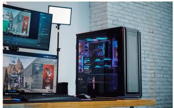
The Enthoo Luxe 2 supports SSi-EEB motherboards, extreme water cooling with dual 480 and dual 360 radiators installed simultaneously and extensive storage with up to x12 HDDs/x11 SSDs. It also features good looks, in anthracite gray or satin black with a minimalist front panel, tempered glass window and integrated RGB lighting (compatible with Asus, Gigabyte, MSI, ASRock and Razer lighting systems).
