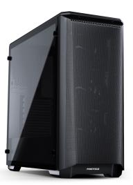
Available with either a fan controller in black and two black fans or an integrated digital RGB controller and x3 RGB fans in black or white, the P400A is built in powder-coated steel with a tempered glass side and a mesh front. The company says the front panel features "an ultra-fine performance mesh that brings the best possible performance while keeping dust from entering the system," together with x2 USB 3.0 ports, mic, headphone, power and reset buttons.
