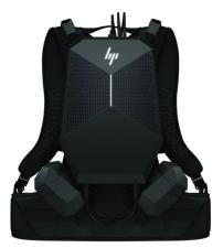
Technically aimed at the enterprise market (HP points out applications such as workplace training and VR development), the VR Backpack G2 still makes an interesting showcase for free-roam VR technology. It carries an 8th generation Intel Core i7 CPU and an Nvidia 2080 GPU to deliver what HP claims are 30% better performance and 25% faster graphics, and is powered by a pair of hot-swappable batteries.
